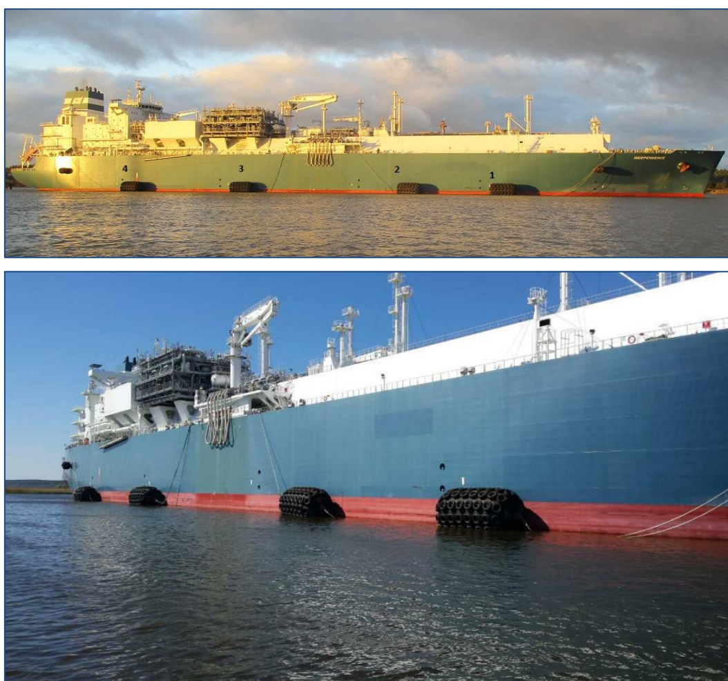
Fig. 61 FSRU ship with "Yokohama" fenders at side of mooring LNG carrier
