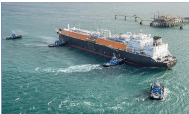
Image 22 Typical use of tag for LNG carriers mooring3
