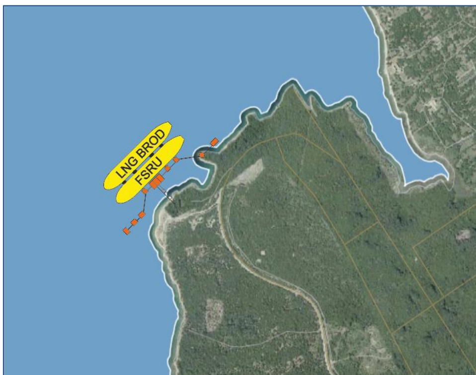
Image 33 Layout drawing of the terminal with the location of FSRU vessel docking place
