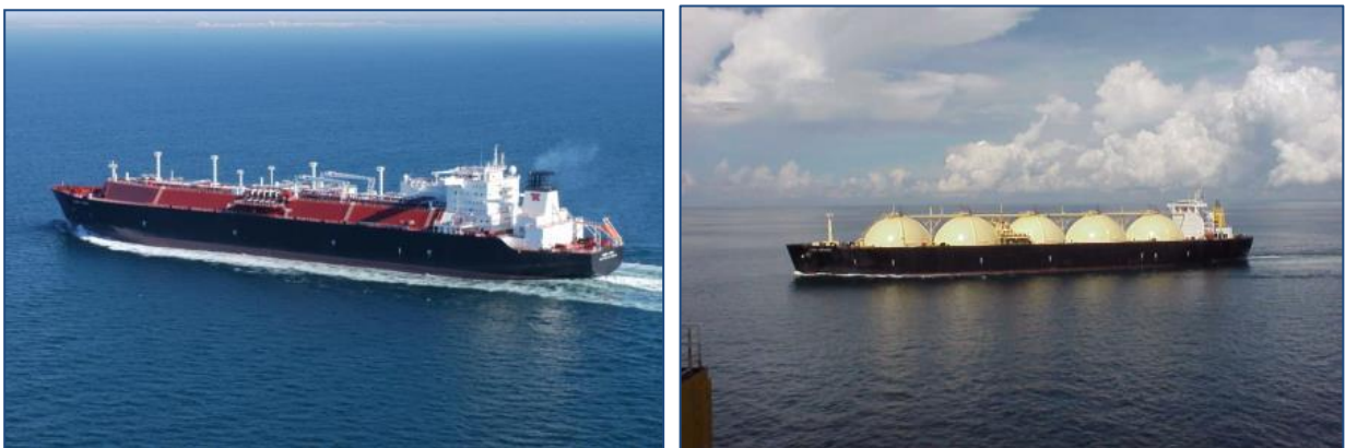
Figure 19 LNG vessel with membrane tanks (left) and self-supporting tanks (right) 2
