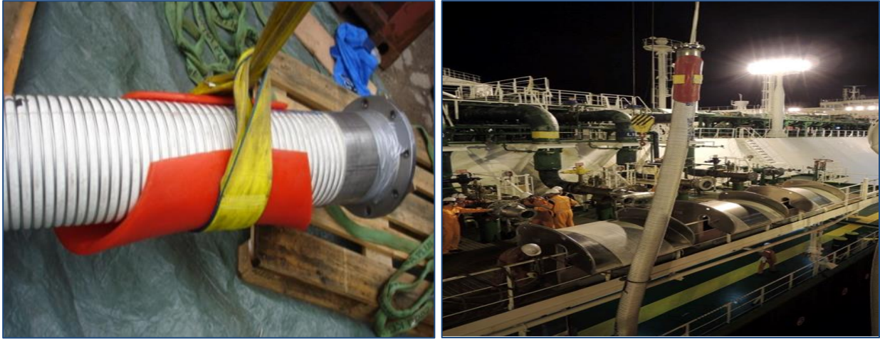
Image 25 Flexible cryogenic cargo transfer hoses handling and tie-up in the saddles.4
