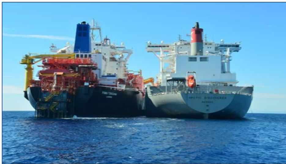
Image 29 Use of fixed type loading arms for offshore cargo operations 5
