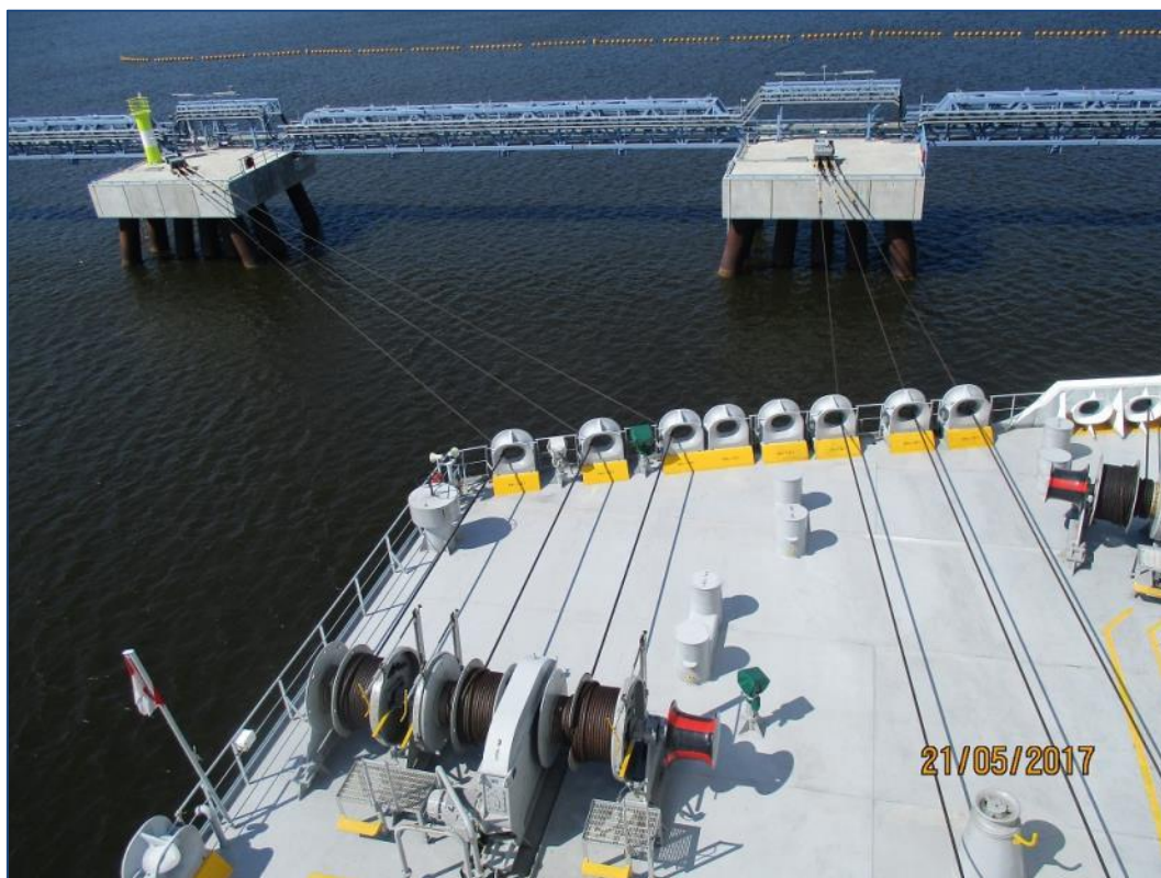
Fig. 64 FSRU ship mooring to solid structure berths
