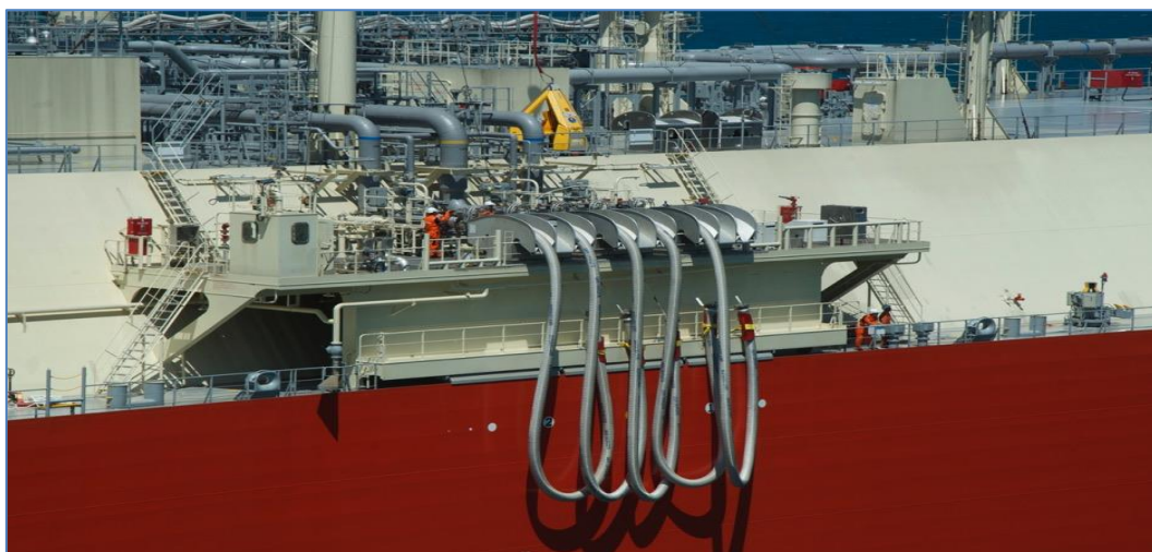
Image 24 Flexible cryogenic cargo transfer hoses on FSRU vessel
