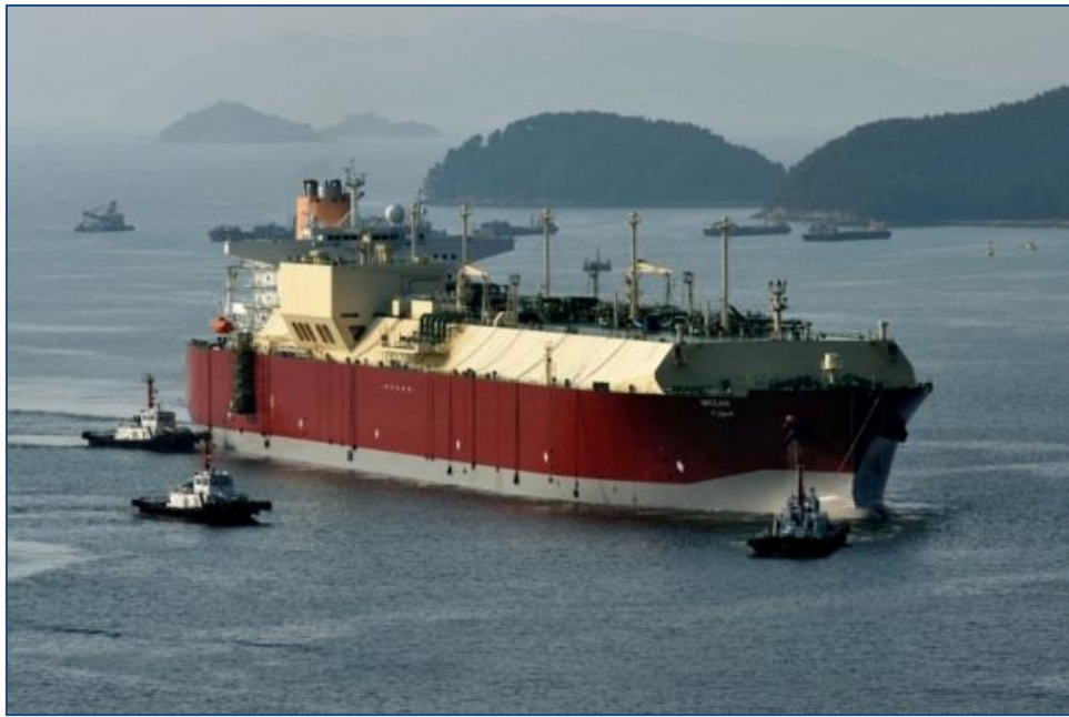
Figure 20 Q-Max LNG vessel during manoeuvring
