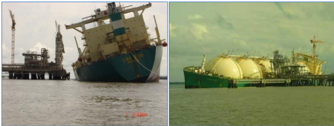
Figure.75 LNG EDO ship list due to irregular ship balancing
